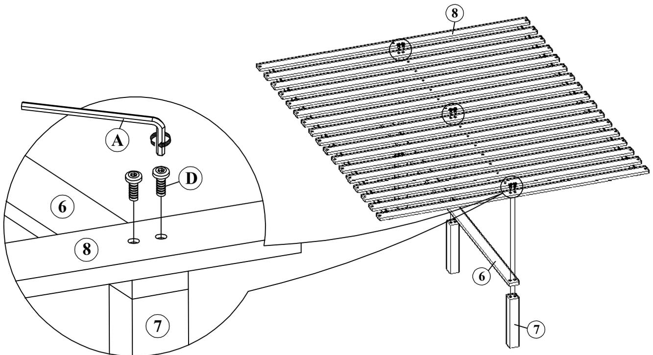
STEP 5 : Attach Assembled Center Support to Assembled Bed with (J) using a Screwdriver as shown.
